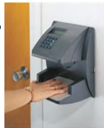
Figure 5-10 A hand geometry system verifies identity based on the shape and size of a person's hand. Courtesy of Ingersoll Rand Security Technologies
