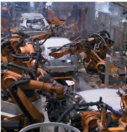
Figure 1-39 Automotive factories use industrial robots to weld car bodies.
