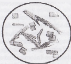
16-rasm. Paxikarpinning kobalt rodanid bilan bergan kristallari
