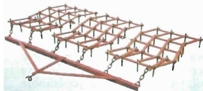
12- rasm. Sixli borona: 1 – borona; 2 – zanjir, 3 – pishang.
