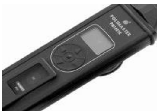
11.3-rasm. PM1401K rusmli \alpha -, \beta -, \gamma -nurlar dozimetri
