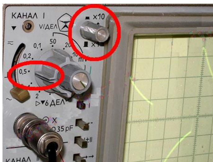
4.21-rasm. C1-83 ossillografida vertikal bo'yicha masshtabni aniqlash.
