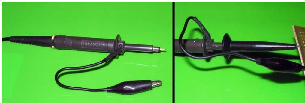
8.6-rasm. Zamonaviy ossillografning shchupi, chapda "ignali", o'ng tomonda qismali.
