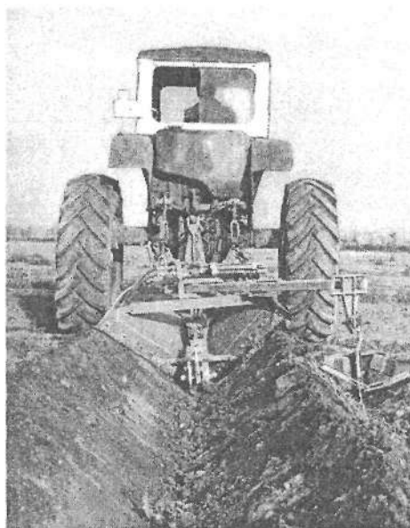
51-rasm. K3Y-0,3 ariqqazgich-tekislagich bilan muvaqqat ariq ochish.
