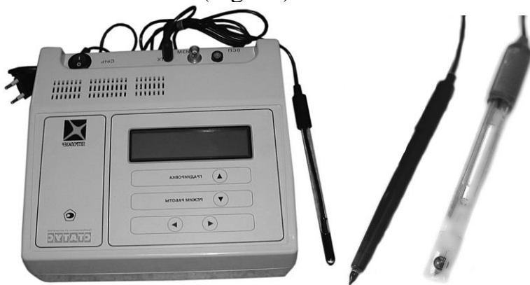
Pic. 24. pH-meter "Status" and combined electrodes to determine the acidity of milk and cheese
