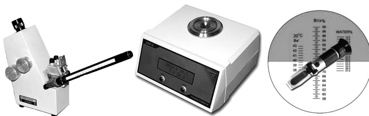
Pic. 56. IFR 454 2VM refractometer, portable refractometer and enlarged scale, digital refractometer ALR-3
