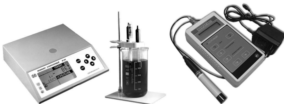
Pic. 58. Universal ionometer "I-160" and nitratometer "Nitrate-test" Reaction recording. The instrument scale readings with the help of a calibration table are translated into nitrate content and compared with the maximum allowable concentrations of nitrates (in mg/kg):
