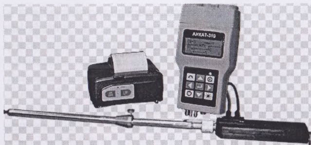
1-rasm. Is gazlarini o'lchaydigan gazoanalizator ANKAT 310
