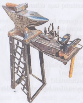
20–rasm. Ko'chma sandon
