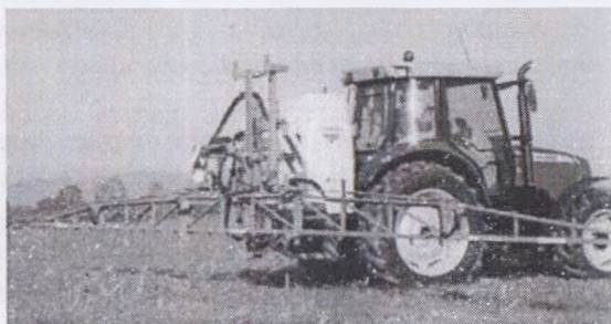
11.3-rasm. Lemken firmasining EvroLux 1200 TLE shtangali purkagichi.
