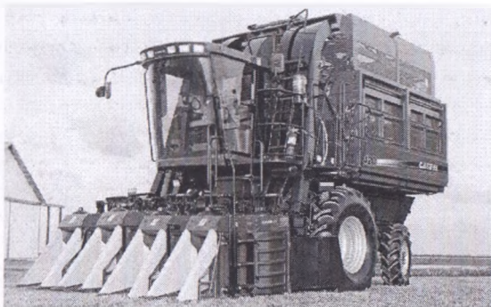
12.1-rasm. “Keys-2022” gorizontall paxta terish mashinasi.
