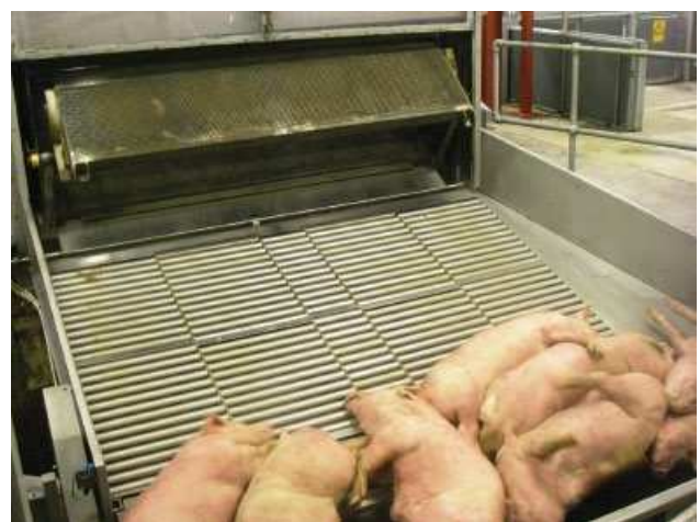
Figure 7.5 CO 2 anaesthesia. Combi-compact system showing convenient shackling position after stunning (Reproduced with permission from David Armstrong).
