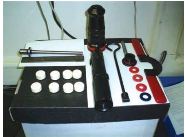
Figure 7.4 Captive bolt pistol, taken to pieces for daily cleaning.
