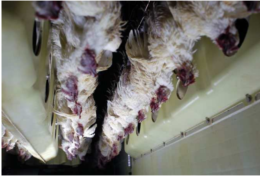
Figure 10.6 Aeroscalding – scalding without immersion into scalding (Reproduced with permission from Stork Poult Processing, Boxmeer, The Netherlands).
