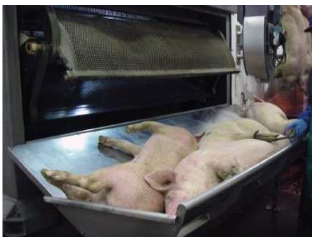
Figure 7.5 CO 2 anaesthesia. Combi-compact system showing convenient shackling position after stunning (Reproduced with permission from David Armstrong).
