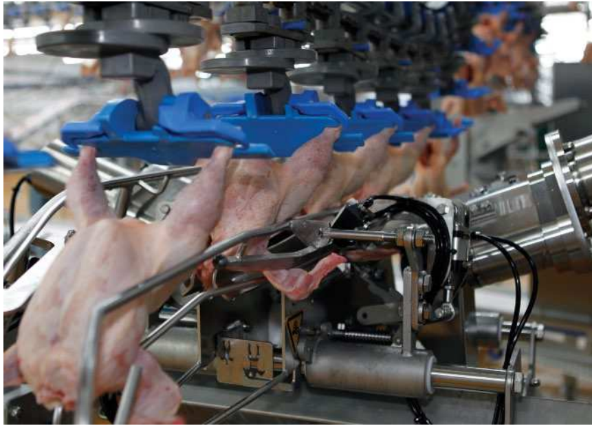
Figure 10.23 Cut-up line – wing processing (Reproduced with permission from Stork Poultry Processing, Boxmeer, The Netherlands).
