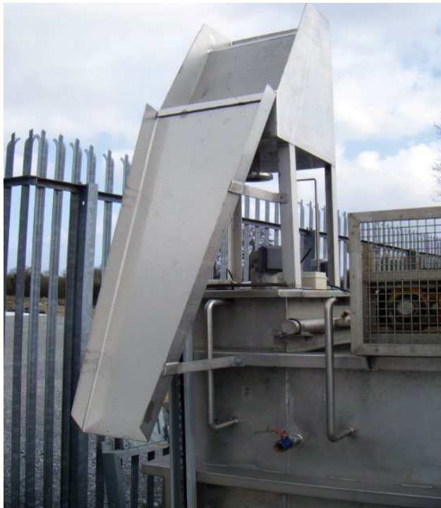
Figure 3.9 Wedge wire rundown screen (by courtesy of Enisca, Cookstown, Northern Ireland).
