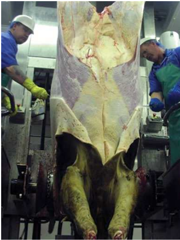
Figure 8.4 Downward hide-puller; more hygienic than upward puller and can also skin head, previously prepared.
