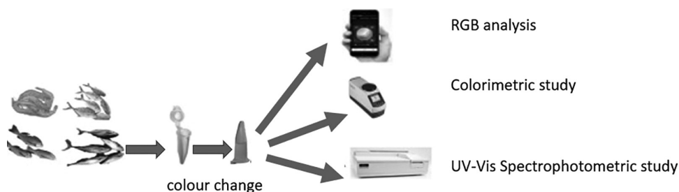
FIGURE 1.6 Use of biodegradable hybrid polymer film for the detection of formaldehyde in seafood products. Reproduced from Rovina et al. (2020) with permission of Elsevier.
