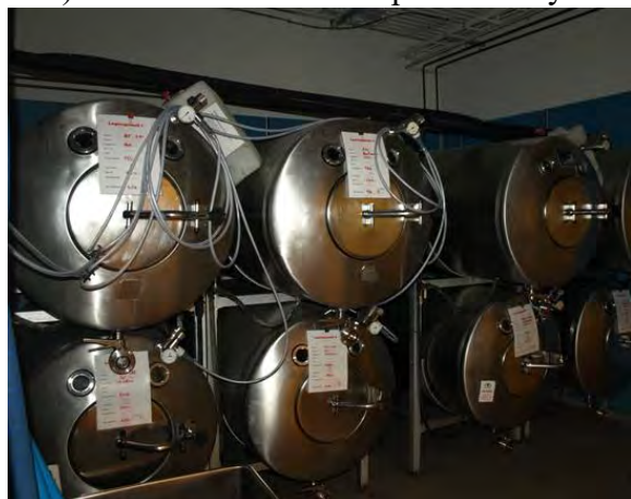
Figure 6.26 The fermentation of grape juice to make wine produces CO 2 as a byproduct. Fermentation tanks have valves so that pressure inside the tanks can be released. (credit: Clark et al. / Biology 2E OpenStax )
