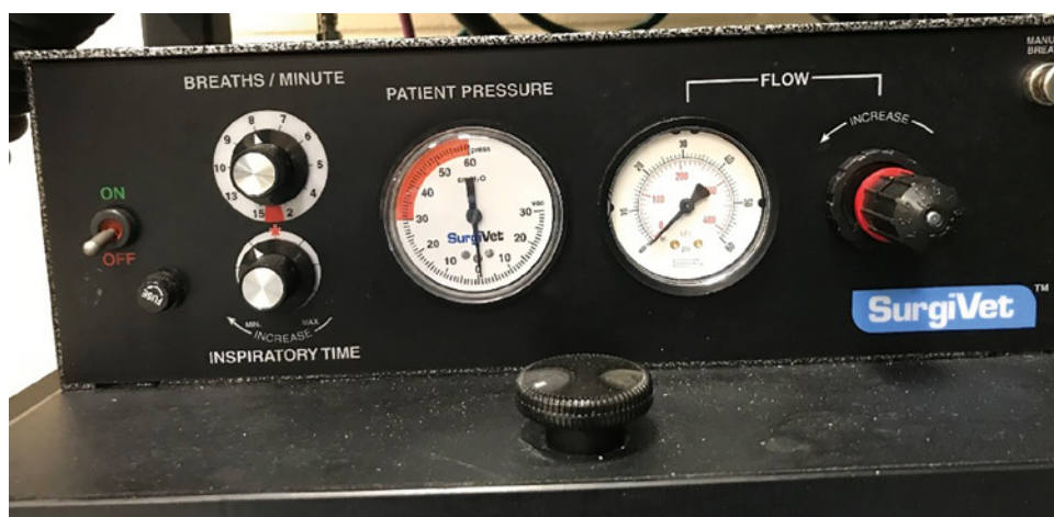
Figure 6.3 Preset respiratory parameters, respiratory rate, tidal volume, peak inspiratory fresh gas flow rate or peak inspiratory pressure, and/or inspiratory to expiratory ratios (I:E ratio) or inspiratory time of a ventilator (SurgiVet).
