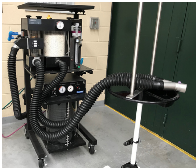
Figure 6.8 Pneumatically powered with electrical control ventilator with rubber breathing system and bellows (SurgiVet).
