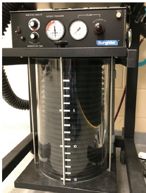
Figure 6.6 Ventilator with hanging bellows for large animals (SurgiVet).
