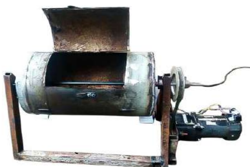
1-rasm. Lichinkalarni qurtish uchun mo‘ljallangan barabanli tajriba uskunasini(0.5 kw/kg).
