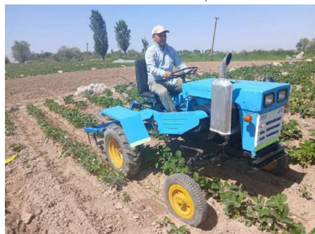
1-rasm. Quvvati 13,4 kw, kengligi 1,40sm, uch labkali qamrov kengligi 1,50smli chizil bilan agregatlangan mini traktor.
