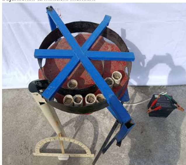
4-rasm. Turli shakldagi stakanchalarning aylanuvchi taglikdagi harakati
