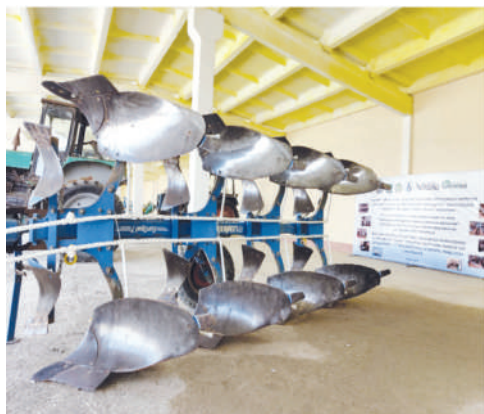
1-rasm. Shudgorlash jarayonida tuproq osti va ustiga biosolvent preparatini sepadigan qurilma.
