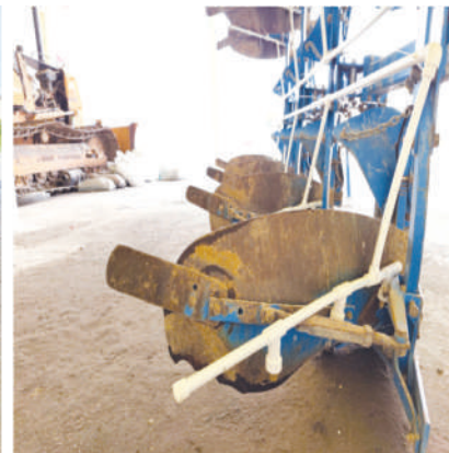
1-rasm. Shudgorlash jarayonida tuproq osti va ustiga biosolvent preparatini sepadigan qurilma.
