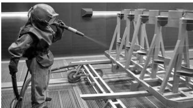
Figure-4. Protection of metal structure from corrosion
