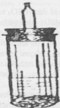
66-rasm. Vodorod olish uchun asbob
