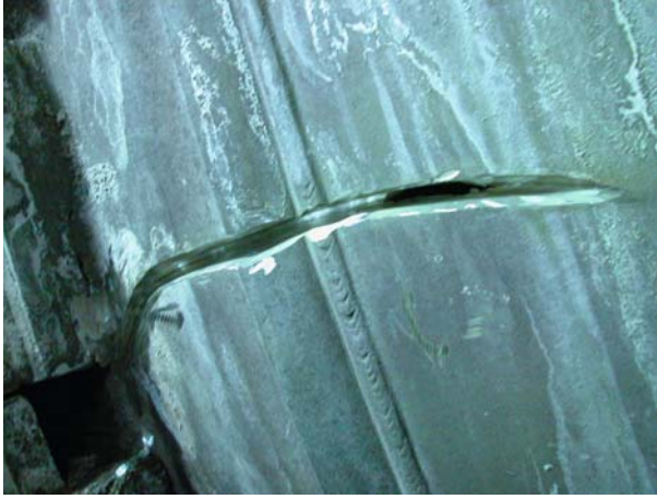
FIGURE 12.3 Thermal stress rupture of an 8.5 foot diameter tube used in a calciner, a device for treating liquid waste and turning it into high-level solid waste.
