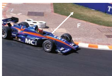
FIGURE 5.21 A car going around a turn has a centripetal force F supplied by the tires.
