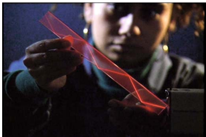
FIGURE 20.20 Total internal reflection in a light pipe.
