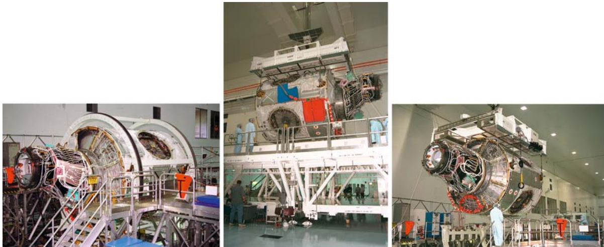
FIGURE 6.10 Node I, a part of the International Space Station, being readied (left) and having its center of mass determined by suspending it from above.
