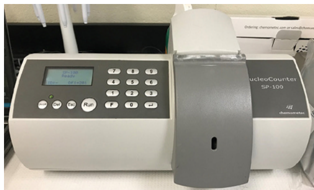
Figure 17.4 NucleoCounter SP-100 (ChemoMetec, Allerød, Denmark). This fluorescent-based counter uses small cassettes loaded with the fluorescent dye, propidium iodide, to determine the sperm concentration (in samples previously exposed to a detergent solution) and percentage of sperm plasma membrane intactness ("viability," in samples exposed to a physiological salt solution).
