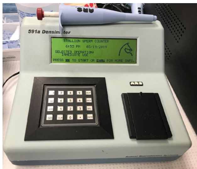
Figure 17.3 Densimeter ("Blue box," Animal Reproduction Systems, Chino, CA) for spectrophotometric determination of semen concentration. This device requires previous dilution of the raw semen with 10% buffered formalin before analysis.
