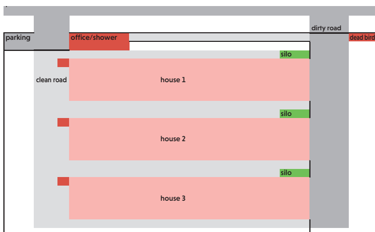
Fig. 13.3: Floor plan of a broiler farm. The clean and dirty roads should be separated. Entry to the house should be via the clean road, while the gate of the poultry house for chick delivery and loading should be via the dirty road. Feed bins and fan-outlets should also be positioned along the dirty road.
