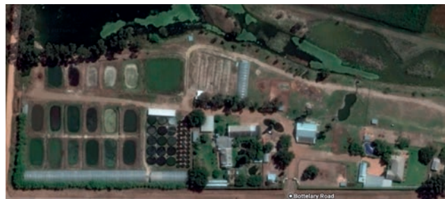
Fig. 19.2 (b): Use of high-resolution satellite imagery (Google Maps) and owner-provided information to delineate aquaculture farm facilities layout: 18 clay ground dams for the rearing of fish; 44 'Porta Pools' for the breeding and rearing of fish; one 100 m greenhouse with 18 breeding and rearing ponds; one 30 m greenhouse with 40 concrete pools for breeding fish; a tropical hatchery housing 500 tanks for breeding, rearing and holding fish; covered display area with a wooden deck and 5 show ponds.
