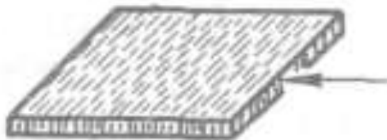
4-rasm. YoPP ni tayyorlashda presslash kuchlarining yo‘nalishi:
