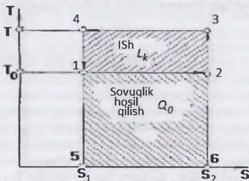
20-rasm . Karnoning teskari (sovutish) tsikli
