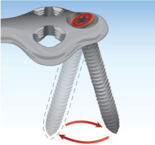
Figure 4.6 Variable angle locking compression plate (VA-LCP) plate combi hole. Four columns of threads in locking hole provide four points of locking between the VA LCP Plate and the specially designed variable angle locking screw. (Source: Modified from Synthes.)
