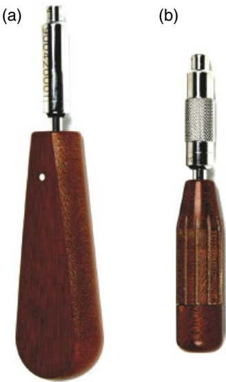
Figure 10.2 Example of a large-handled driver (a) compared to a palm-sized (b). The former should be used with the PAX system to help ensure adequate insertion torque is generated by hand.
