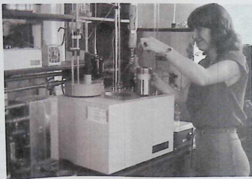
Fig. 7.9. A bomb calorimeter used in the determination of the calorie content of feeds. The bomb (the container in which the feed sample is burned) is in the technician's right hand. The feed sample is put into a cup in her left hand and then inserted into the bomb. (Courtesy of OSU Rabbit Research Center)
