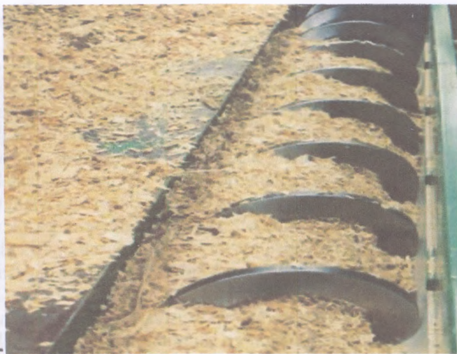
11.1-rasm. Spiral – vintli (shnekli) transporter.
