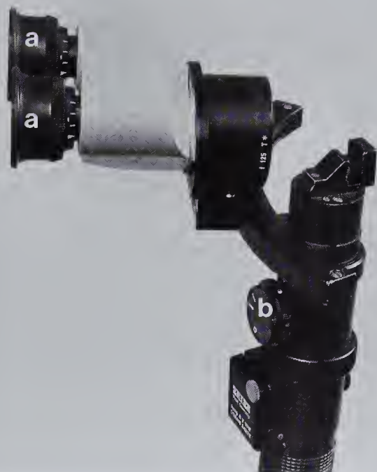
Fig. 20.8 A handheld Zeiss biomicroscope. Note the moveable eye pieces (a) and light control dial (b).
