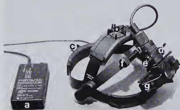
Fig. 20.9 A Heine Omega 200 indirect ophthalmoscope. Note the rechargeable power pack (a), circumferential headband adjuster (b), the vertical headband adjuster (c), the light aperture size lever (d), the light filter control lever (e), the control knob for angulation of the eyepieces (f), and the teaching mirror viewing ports (g).
