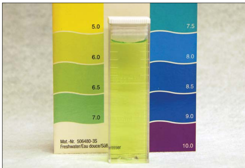
Figure 2.1 Water sample tube (center) with pH color comparator chart. (TetraTest, Spectrum Brands, Blacksburg, VA.)
