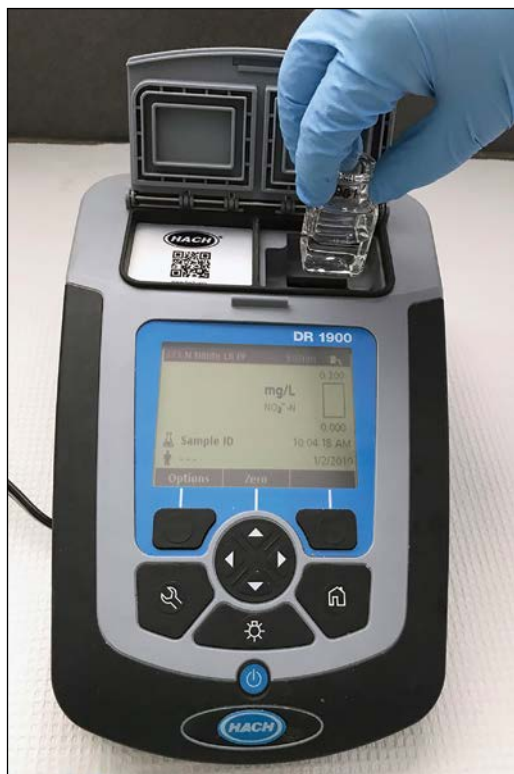
Figure 2.4 Spectrophotometer for water analysis. (HACH Company, Loveland, CO.)
