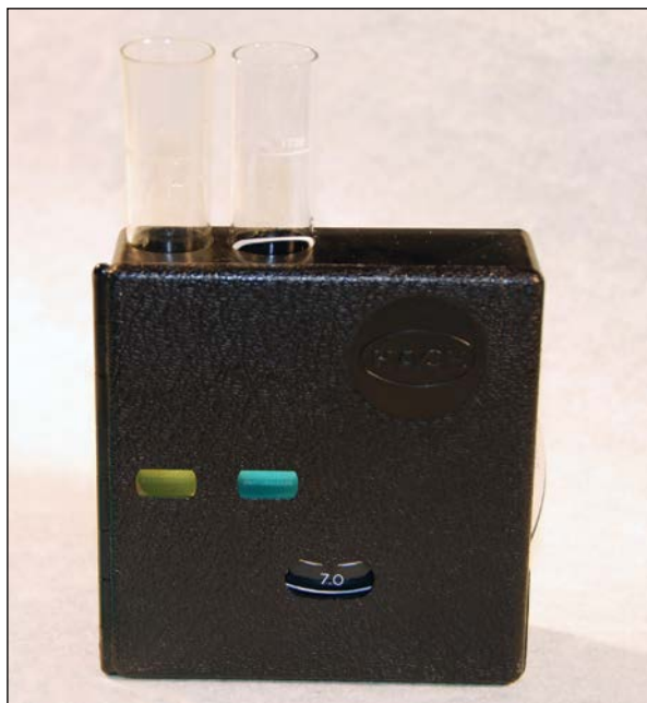
Figure 2.5 Standard blank (right tube) and test sample (left tube) color comparison method with pH color disk. (HACH Company, Loveland, CO.)
