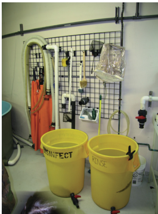
Fig. 6.3 Example of dedicated equipment for servicing a quarantine facility or system. Note the easily accessible disinfectant and rinse containers, drying racks for cleaned and disinfected equipment, and dedicated coveralls for the quarantine facility.
