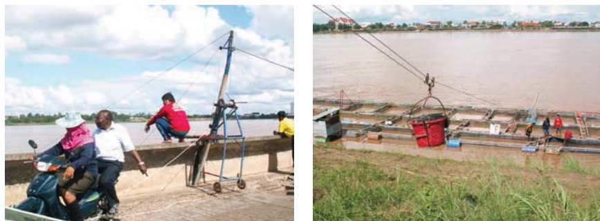
Fig. 9.4. Tilapia harvesting from cages lifting by using pulleys and metal strings connected to a motorbike engine.
