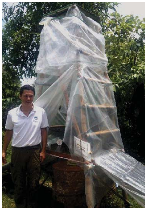
Fig. 4.9. Simple drier that can work with solar power and/or firewood.
