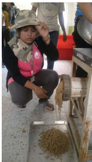
Fig. 4.10. Making fish feed (sinking) pellets using simple mincer.
