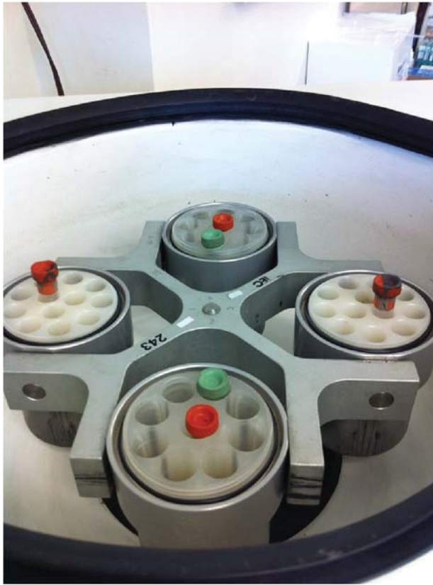
Figure 1.3 Balanced centrifuge. The same sample weight is placed on opposite sides of a centrifuge rotor to balance the sample load during centrifugation. This prevents damage to the rotor.
