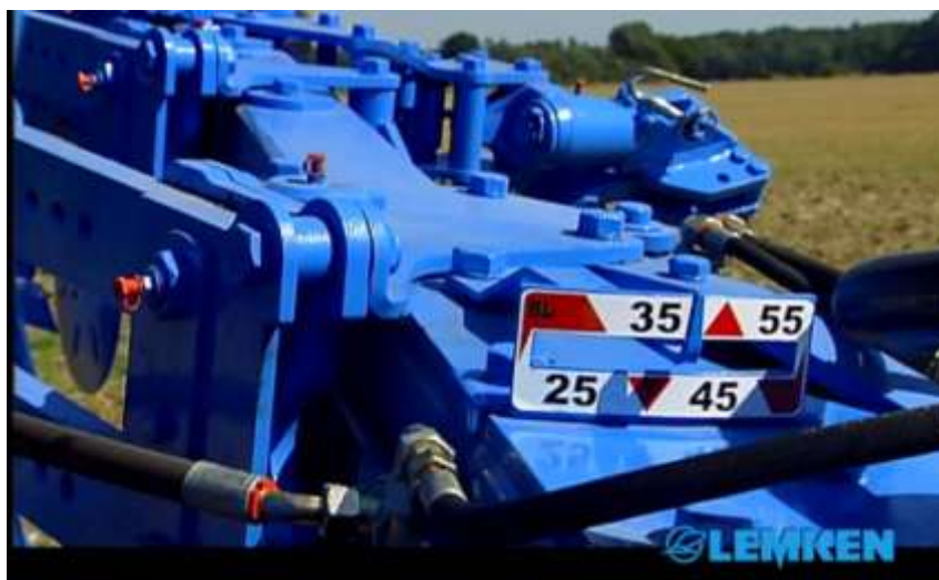
35-rasm. Lemken firmasi plugining qamrash kengligini o‘zgartirish innovatsion qurilmasi
