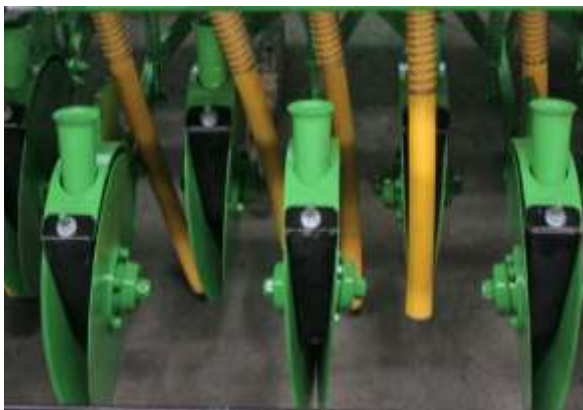
39-rasm. Don ekish seyalkasining mexanizmlari
