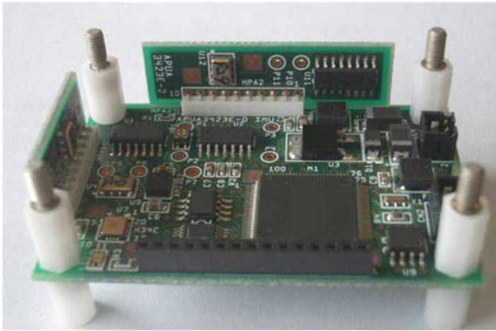
Fig. 11.2 Overview of small attitude sensor
