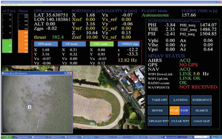
Fig. 12.6 The interactive interface of the ground control station during vision-based autonomous hovering
