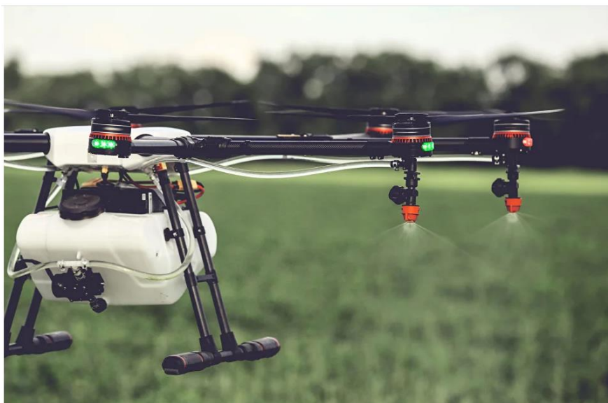
2.10-rasm. GPS qurilmali dronga o'rnatilgan purkagich
