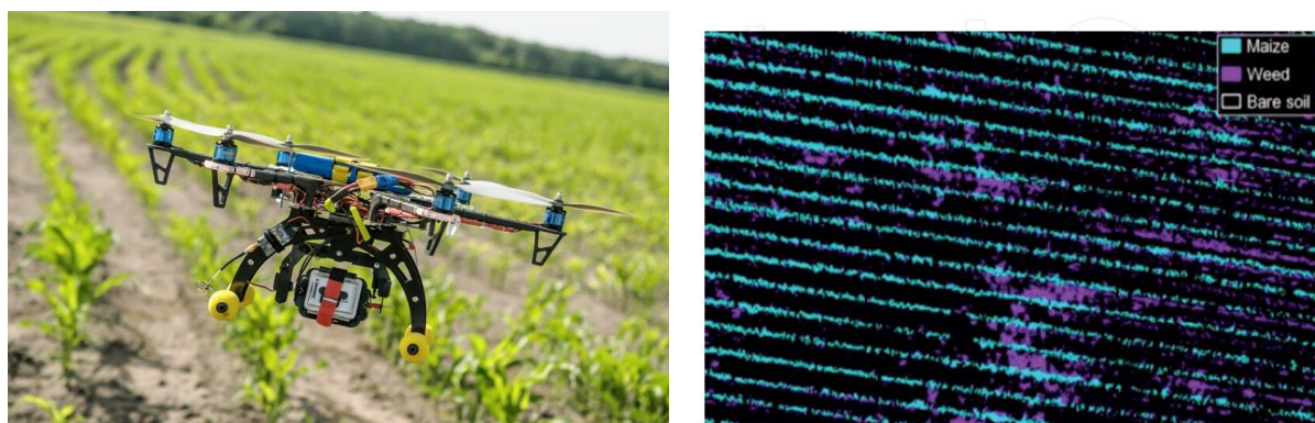
7.11-rasm. Dron yordamida makkajo‘xori dalasini tasvirga olish (a) va dalaning ko‘rish va yaqin infraqizil diapazondagi tasviri (b)
