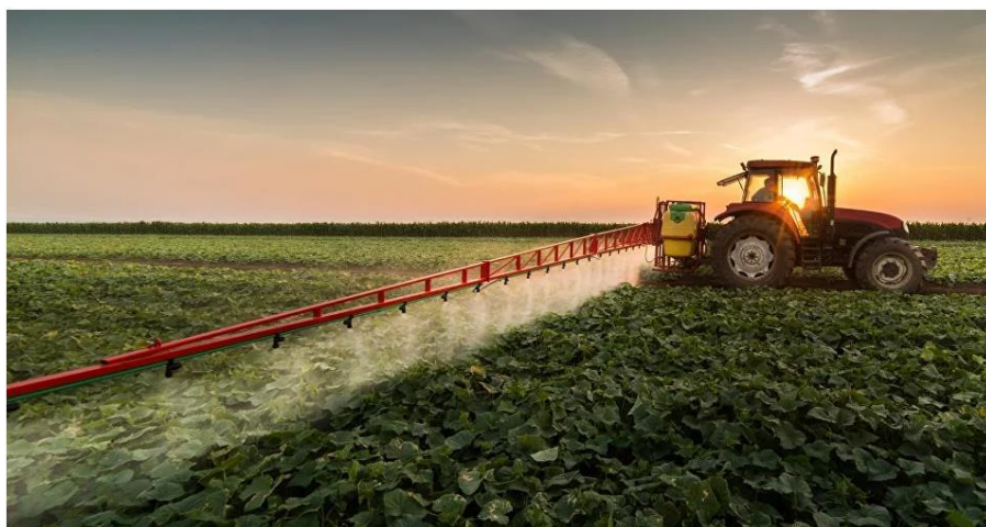
2.9-rasm. GPS qurilmali traktor bilan agregatlangan purkagich
