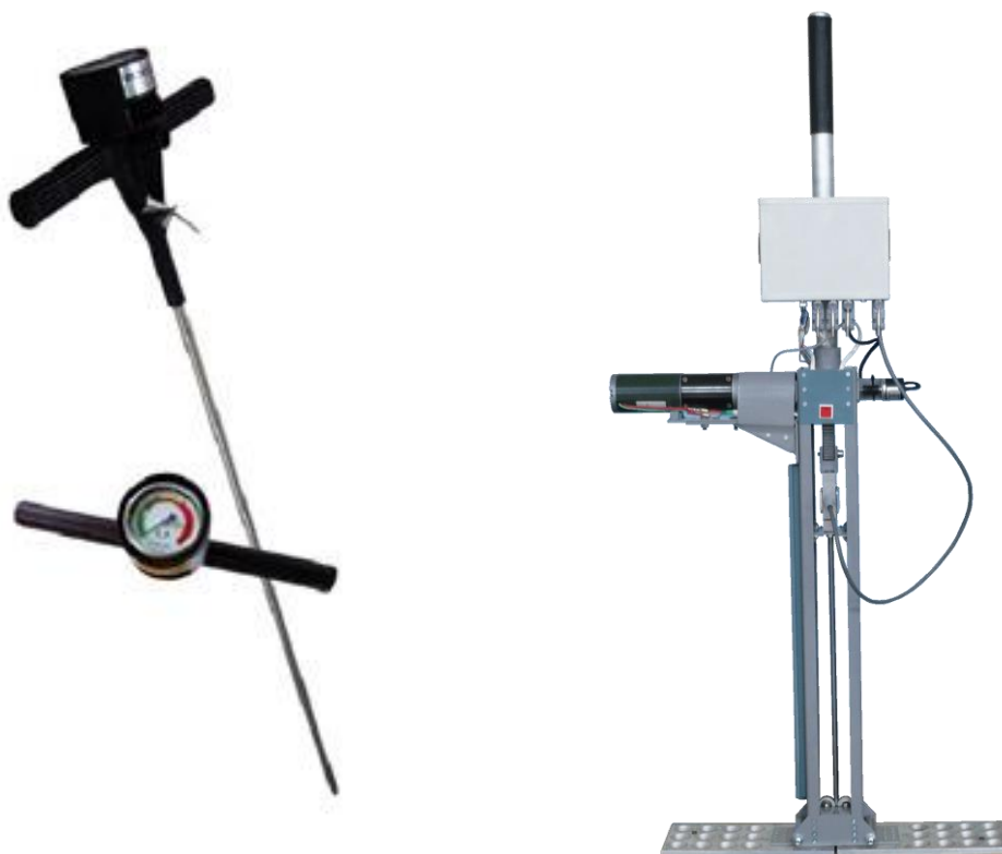
6.11-rasm. Tuproq qattiqligini o‘lchash asboblari
