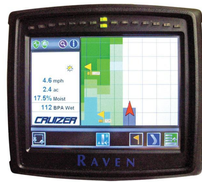
9.19-rasm. Raven firmasining hosildorlikni oniy aniqlash tizimi monitori
