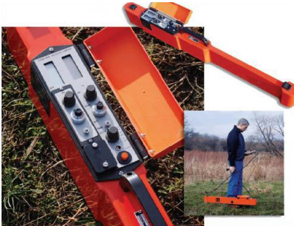
6.16-rasm. Tuproqning elektr o'tkazuvchanligini skanerlash
