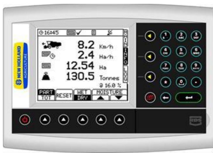
9.17-rasm. New Holland kombaynlarining hosildorlikni lahzalarda aniqlash tizimining monitori
