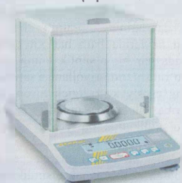
3-rasm. Analitik tarozi Kern ABS 220-4N
