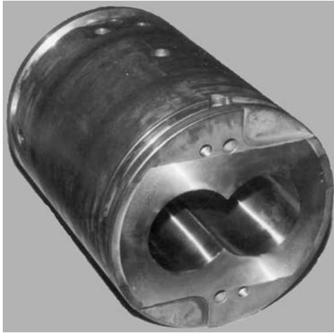
Figure 15.6 Cross-section of the barrel of a twin-screw extruder. (Courtesy of Clextral)
