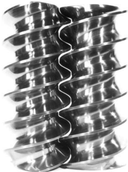
Figure 15.8 Intermeshing twin screws. (Courtesy of Clextral)
