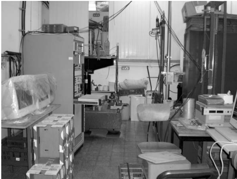
Figure 26.2 Vibration tables in a packaging research laboratory. (Courtesy of the Department of Biotechnology and Food Engineering, Technion)
