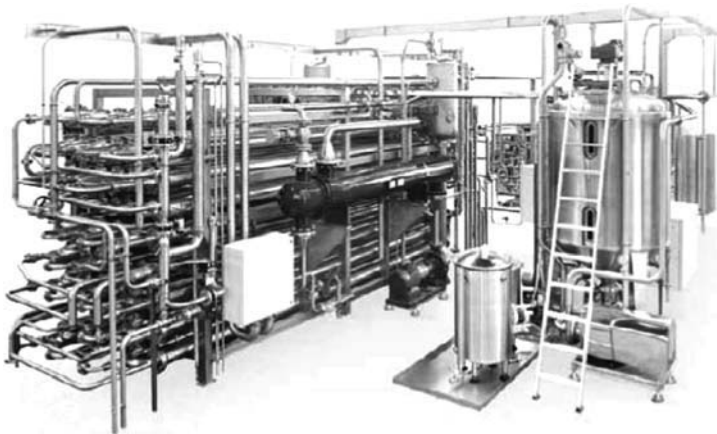
Figure 3.14 Tubular heat exchanger assembly in aseptic processing plant. (Courtesy of Rossi & Catelli)
