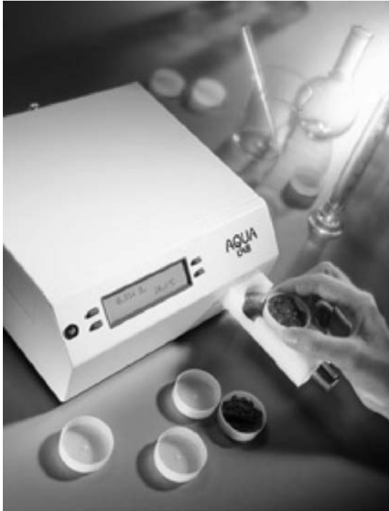
Figure 1.4 Measurement of water activity
