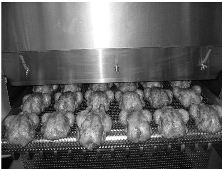
Figure 24.5 Continuous roasting of chicken. (Courtesy of FMC FoodTech)
