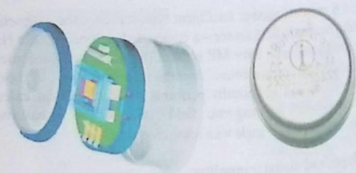
Figure 6.5 The temperature sensor iButton of the Dallas Semiconductor (Dallas Semiconductor 2005) (permission of Dallas Semiconductor)
