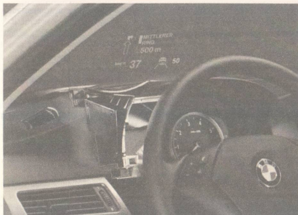
Figure 13.37 BMW HUD – a clear information source – albeit in German here! (Source: Siemens)
