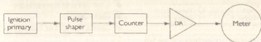
Figure 13.8 Block diagram of a tachometer which uses signals from the ignition coil
