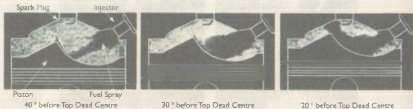
Figure 10.28 Behaviour of fuel spray (injection in compression stroke) - Schlieren photo method
