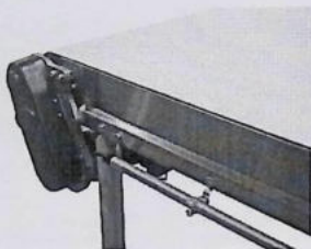
FIGURE 26.33 Motors should rather be located below the line of the product flow. Gears, chains and motors of belt drives must be covered to avoid any contamination of product. However, a chain guard (essential from an occupational safety point of view), when open, may provide a place where product may accumulate, allowing microbes to multiply to large numbers and so posing a contamination risk for the food product on the belt. Courtesy of Dornier Conveyors.
