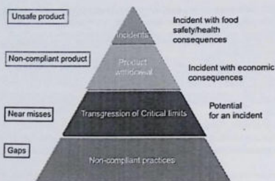
FIGURE 37.4 Every failure can be a potential for an incident. Monitoring the failures, understanding their cause, communicating and acting upon them as early as possible can reduce the risk of incidents.
