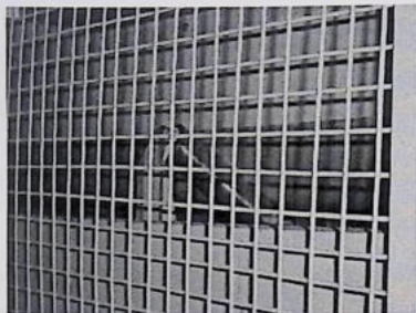
FIGURE 26.37 Example of a hygienically designed guard. Courtesy of P.T. Group.
