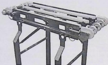
FIGURE 26.31 Conveyor frames should have an open structure without horizontal surfaces and with a minimum of hidden areas/surfaces. At the outside, the framework consists of vertical plate members positioned longitudinally, which also serve as a lateral belt guide. The conveyor frame is an all welded construction with solid round cross-members, welded at the outside framework. The use of bolts and nuts for fastenings is reduced to a minimum. The cross-members not only act as structural frame members, but also as belt supports. The weld-on flat cross-members are provided with gaps to accommodate the freely located plastic wear strips that help to support the conveyor belt. No bolts, holes or nuts were used for fastening the ultra-high-molecular-weight (UHMW) polyethylene wear strips. To minimize cleaning time, these belt supports are easily lifted out of the frame by means of a quick tension-release arrangement and without manual tools. The cut-outs in the frame allow spraying and cleaning of the inside of the conveyor without lifting the belt. The conveyor shown is provided with a swivel-mounted roller that releases tension, providing improved access to the space between belt and bearing strips for cleaning and disinfection. The frame member closest to the point where the belt runs onto the drive roller sprocket also serves as a guard. Stand-off legs keep fasteners out of the food zone. Courtesy of Dornier Conveyors.
