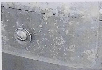
FIGURE 26.3 Product contact surfaces of this equipment are not readily accessible for manual cleaning and disinfection. Moreover, the dome screw with drive slot and washer creates gaps and crevices where debris collects. Courtesy of Joe Stout, American Meat Institute.
