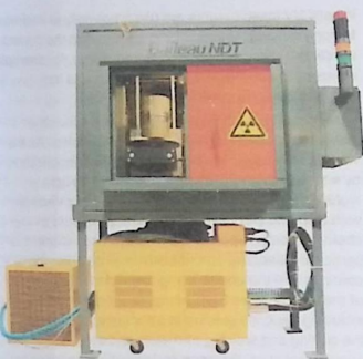
Figure 14.9 X-ray generator cabinet
