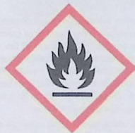
Danger Extremely Flammable Gas
