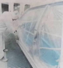
Figure 13.13(c) Paint-spraying inside a special room with general ventilation to remove fumes
