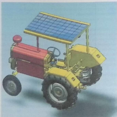
Figure 4. Schematic diagram of solar powered tractor [18].
