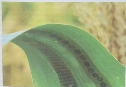
Figure 7. Graphene sensors on plant leaf to sense water transpiration and measure plant water to control irrigation.
