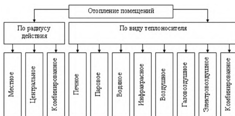
Fig. 1. Classification of heating systems
