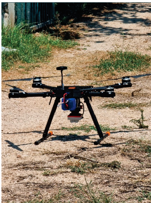
Figure 4. Quadcopter “Mera” (UcanDrone S.A., Koropi Attica, Greece) with the attached multispectral camera, MicaSense RedEdge MX (AgEagle Aerial Systems Inc., Wichita, KS, USA).
