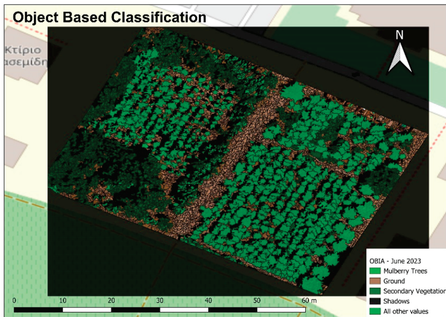
Figure 6. Classified output of the Object-Based Classification for the airborne data of the 28 June 2023 flight.
