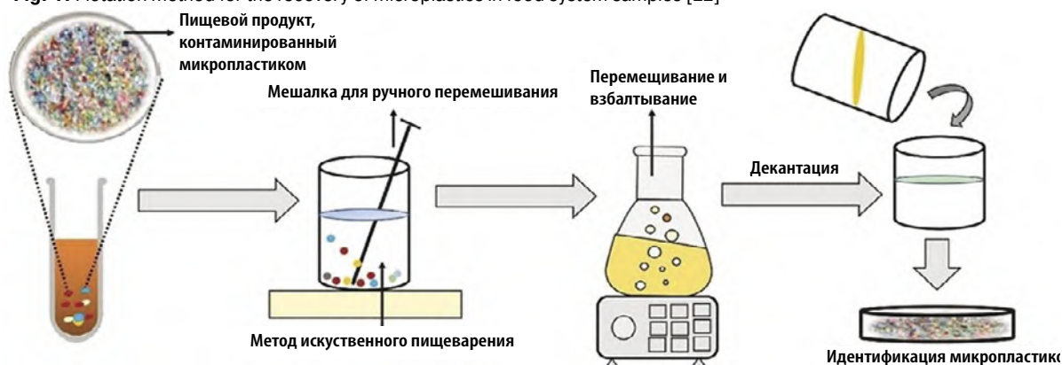
Fig. 1. Flotation method for the recovery of microplastics in food system samples [22]
