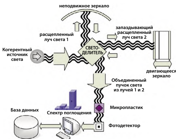
Fig. 5. Schematic diagram of common FTIR analysis modes [68]
