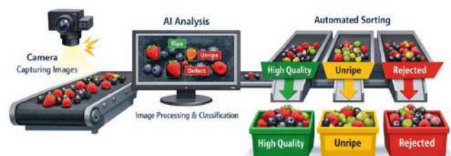
Fig 1. AI-based berry sorting system
