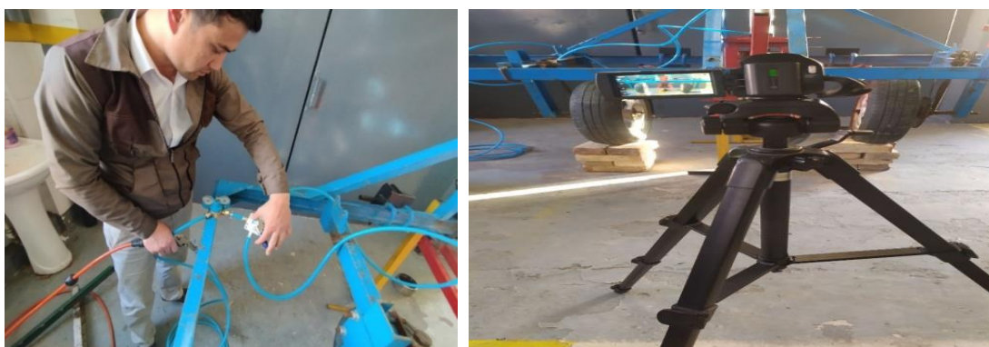
3-rasm. Havo bosimini o'lchash (a) va ishchi organ harakat tezligini aniqlash (b)
