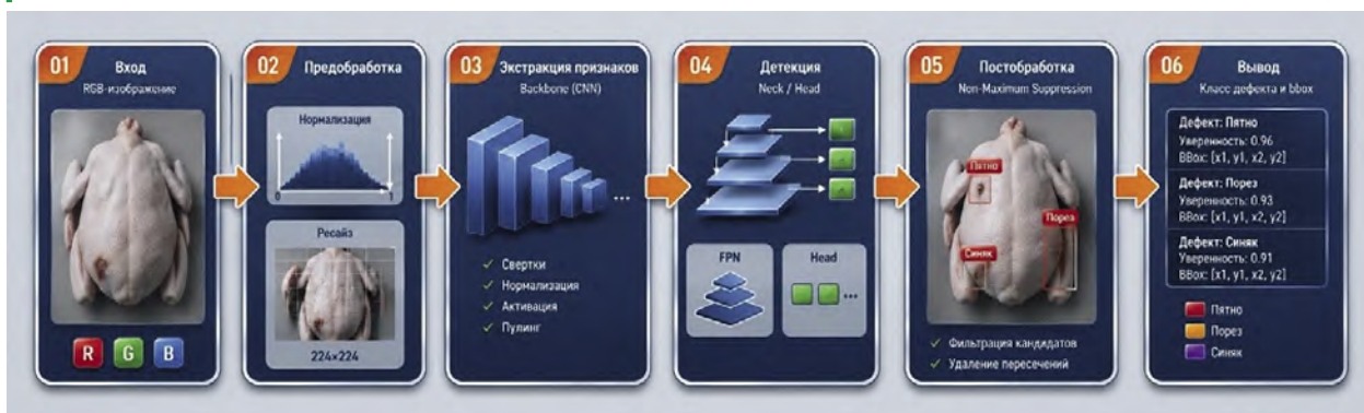
Fig. 1. Image processing circuit
